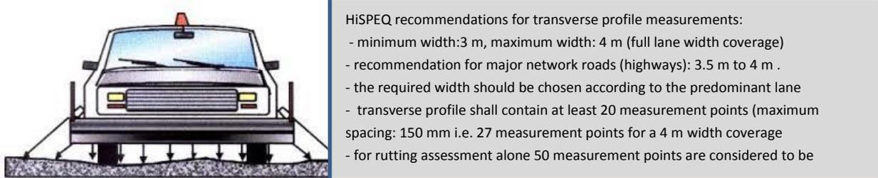
Figure 1 Example HiSPEQ recommendations for specifying transverse profile measurement
